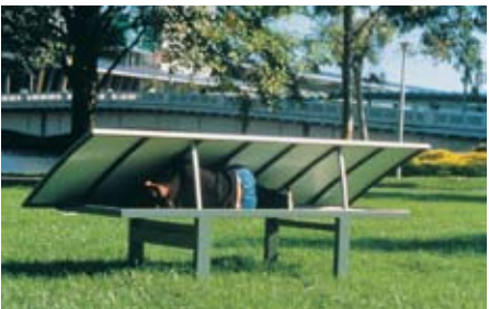
Park Bench House provides basic shelter by converting seats that are used in the day to a shelter at night
